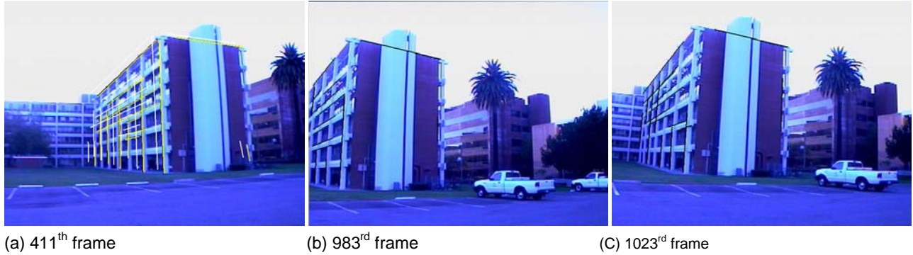
Figure 5 – Snapshots for the line detection. Black lines are the lines detected on the current image. (a) 411 th frame: The white lines detected on the previous image are far from their correspondents on the current image due to large image displacements. The lines (black) on the current image are detected accurately due the accurate prediction (yellow lines) by affine transform. (b) 983 rd frame: Some lines were lost due to the change of viewpoint. (c) 1023 rd frame: The lost lines reappeared and were detected accurately.
