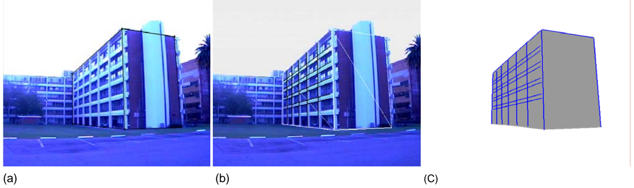
Figure 4 – Snapshot for initialization. (a) The cube (black) specified by the user (b) The manually specified 2D lines (black) on the surface of the cube (white). The white cube is the 3D model inserted into the image. (c) The recovered 3D model for the cube (gray) and the lines (blue) on the surface.
